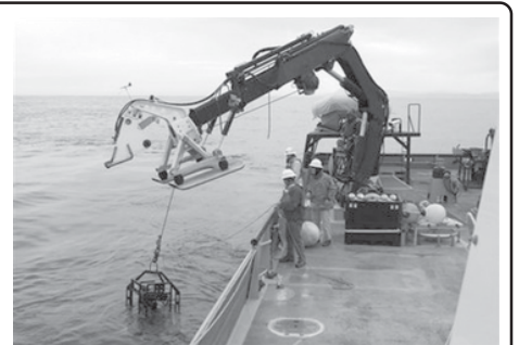
The 502-pound deep sea video camera 'Eye-in-the-Sea' aboard the Research Vessel Point Lobos, is lowered into the Pacific Ocean 22 miles off the California coast. The Eye-in-the-Sea is the world's first Web camera that will offer a window into the darkness of the deep ocean.
