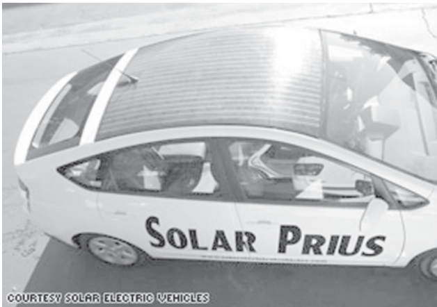
Solar Electric Vehicles in California makes a roof-mounted solar panel for a standard Toyota Prius.—INTERNET
