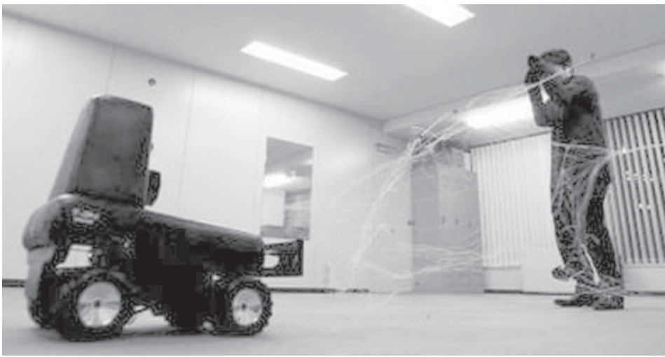
T-34, a remote-controlled security robot, launches a net at a mock intruder during a photo opportunity in Tokyo on 21 Jan, 2009. T-34 users can see live images from the robot's camera and control the robot using a mobile phone. —INTERNET
