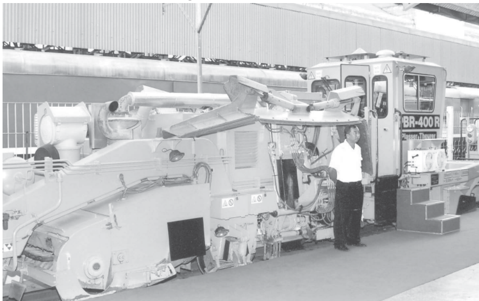
Indian-made profile ballast regulator.
