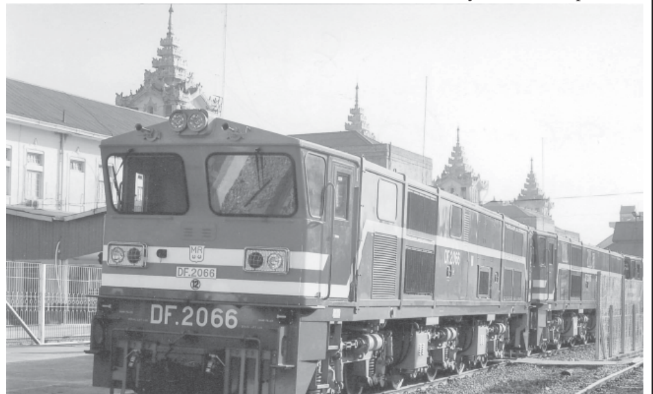
The Chinese-made 2000 HP diesel locomotive.
