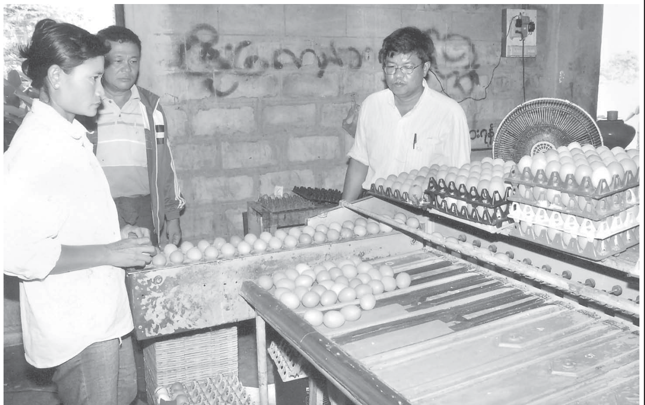
Eggs are categorized in size with the use of the weighting machine.
