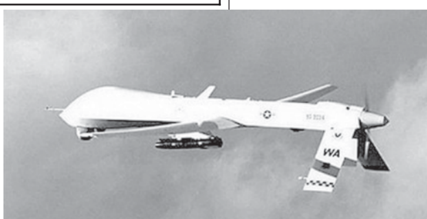
This US Air Force file photo shows an unmanned Predator aerial vehicle with a Hellfire missile attached to it.
