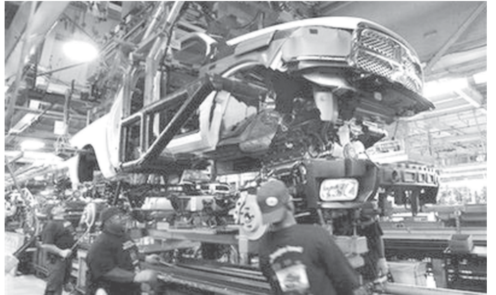
Assembly line workers join the cab to the chassis of Chrysler's new 2009 Dodge Ram pickup being assembled at the Warren Truck Plant in Warren, Mich, on 12 Sept, 2008.—INTERNET
