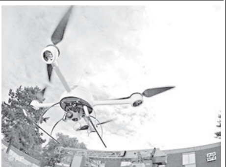
Is it a bird, is it a plane? No, it’s a drone designed to measure the concentration of deadly gases in the air. The project called Airshield was presented in Dortmund. A whole swarm of such drones would be deployed in the event of a major fire or other disaster to sample the air.
