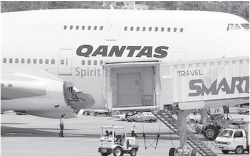
An airline mechanic looks at the damaged right wing fuselage of a Qantas Airways Boeing 747-400 passenger plane following an emergency landing at the Ninoy Aquino International Airport on 25 July, 2008 in Manila, Philippines. The plane, with 350 passengers and 19 crew, was enroute to Australia from London when a loud bang punched a hole in the right wing fuselage, passengers said.—INTERNET
