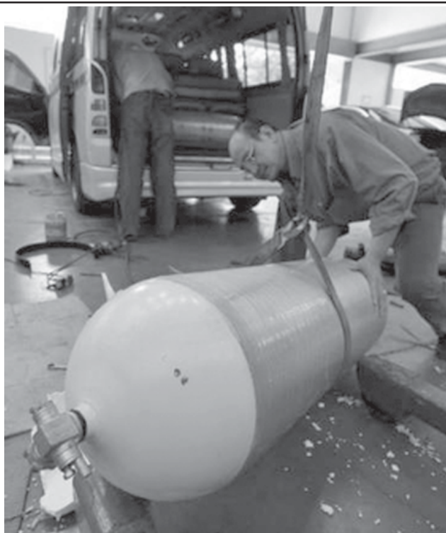
A mechanic installs a bottle of compressed natural gas into a vehicle at a garage in Bangkok on 27 May, 2008. —INTERNET
