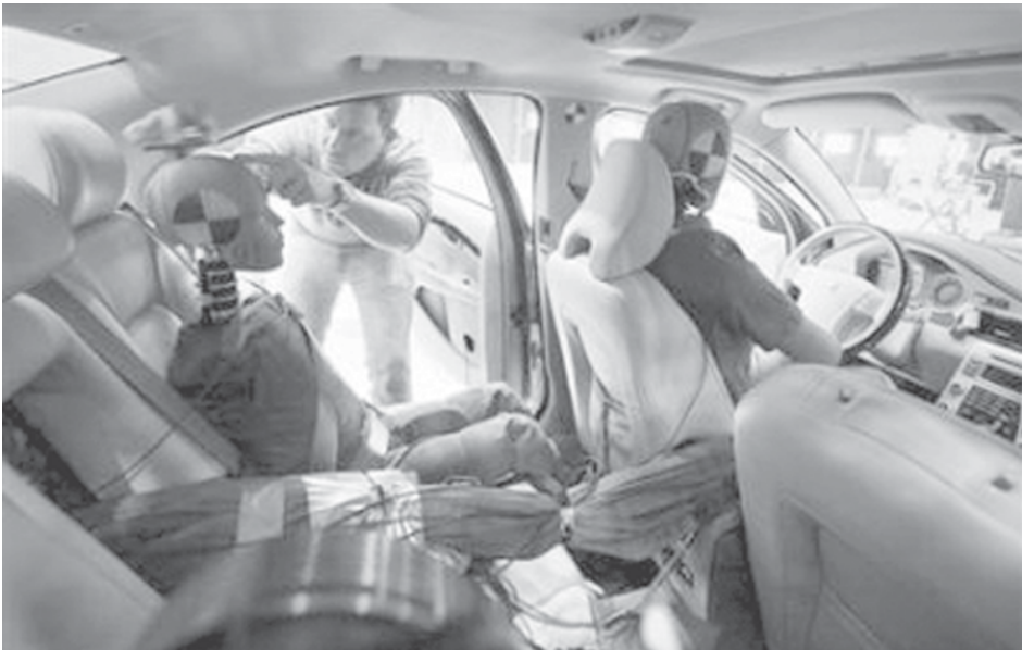
Hampus Olsson, an analysis engineer, checks a test dummy before a crash at the Volvo Safety Centre in Gothenburg recently. The destruction of the orange sedan with its slapdash paintwork may have been intentional but it was far from wanton. It was all part of Volvo's bid to create an injury-proof car by 2020.—INTERNET
