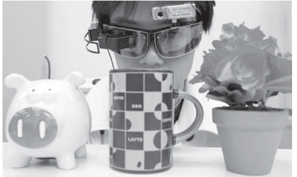
Tokyo University graduate student Hideki Nakayama looks at a mug while wearing "AI Goggles", which is equipped with a web camera and a head-mounted display, during a demonstration at his university's laboratory of the Information Science and Technology in Tokyo on 31 March, 2008. —INTERNET
