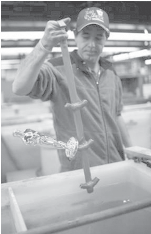
Manuel Nunez works on plating an Oscar statuette on the RS Owens factory floor in Chicago on 11 Jan, 2008. The company will manufacture approximately 75 Oscar statuettes using a 15-step process over a six-week period. The finished statuettes are made of a metal Britannia pewter alloy and are plated with copper, nickel, silver and 24-carat gold. The 80th Academy Awards are scheduled to take place in Hollywood on 24 Feb, 2008.—INTERNET
