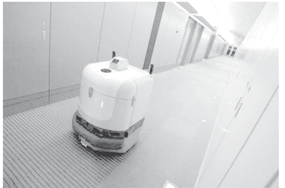
Fuji Heavy Industries Ltd's cleaning robot RFS1 is pictured at an office building in Tokyo recently. It looks like a washing machine on wheels, but the bulky contraption vacuuming the hallways of a Tokyo high-rise is a robot.
