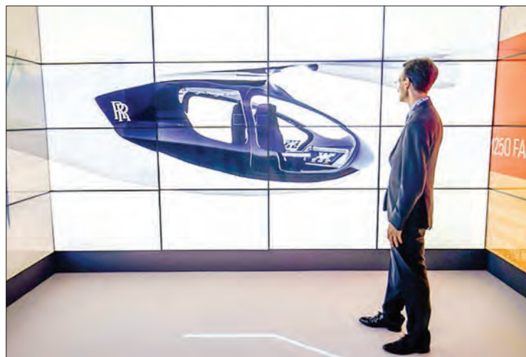
The Rolls-Royce EVTOL plane will seat four or five people, with a flying range of 500 miles (805 kilometres) and a top speed of 200 miles per hour. PHOTO: AFP
