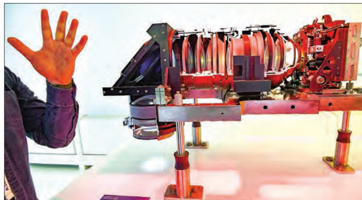
A lens used in the manufacturing of semiconductors at Dutch company ASML, whose latest systems project blueprints of circuitry onto silicon wafers. PHOTO: AFP
