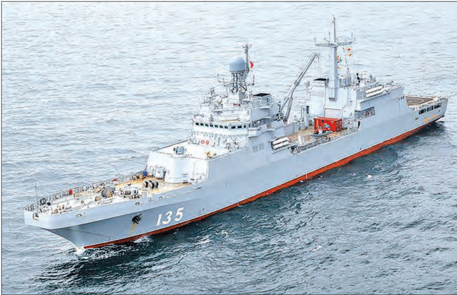
The warship can carry 13 main battle tanks or 36 armoured personnel carriers, or up to 300 marines. PHOTO: TASS
