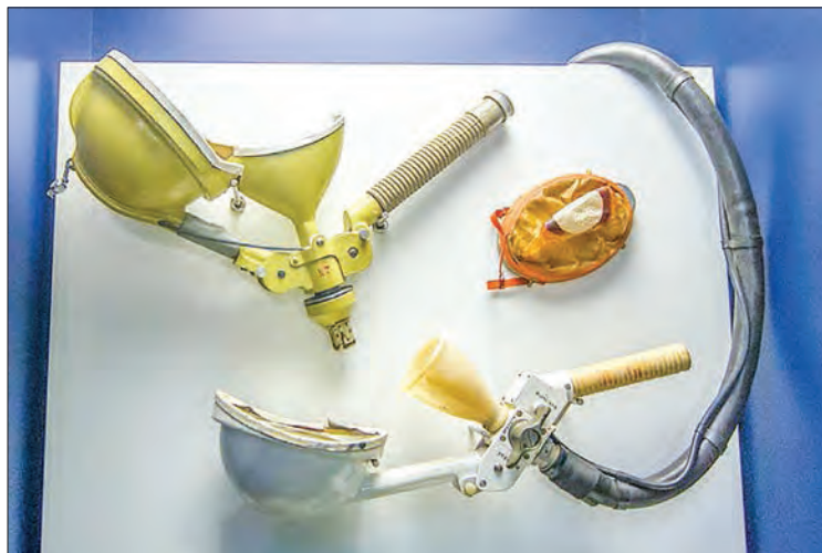
Toilet used on the ISS's Soyuz spacecraft.
