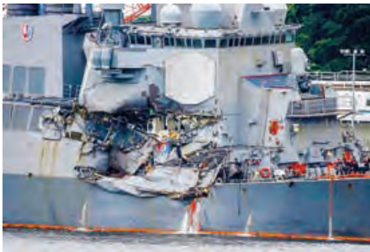
The Arleigh Burke-class guided-missile destroyer USS Fitzgerald, damaged by colliding with a Philippine-flagged merchant vessel, is seen at the US naval base in Yokosuka, Japan. PHOTO: REUTERS
