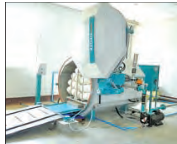
The Yarn Steaming machine. PHOTO: MINISTRY OF INDUSTRY
