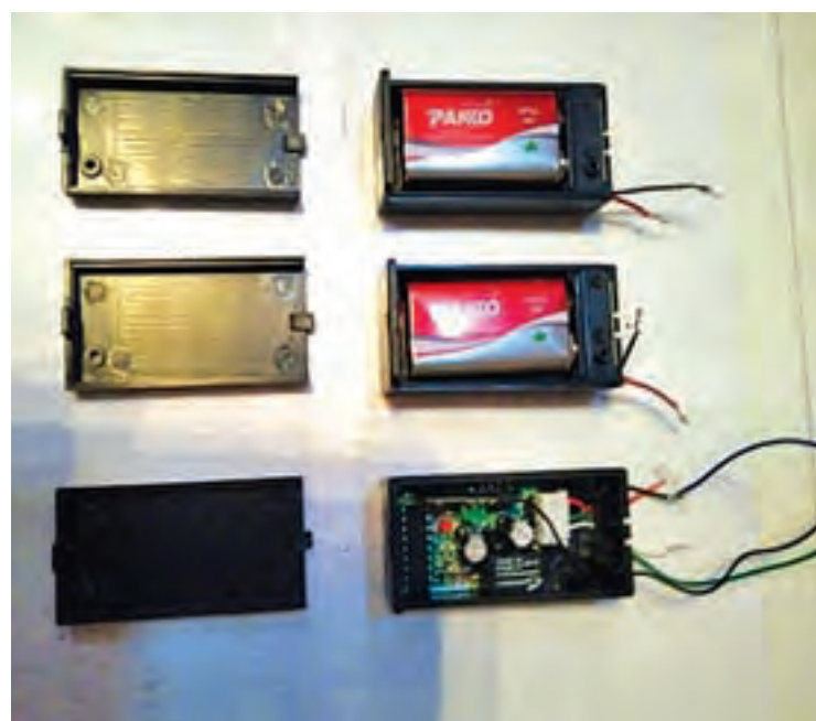
Time control devices linked to 207 mm launcher rockets.
