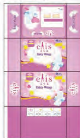
Fig. 7 - Reduced Development View
