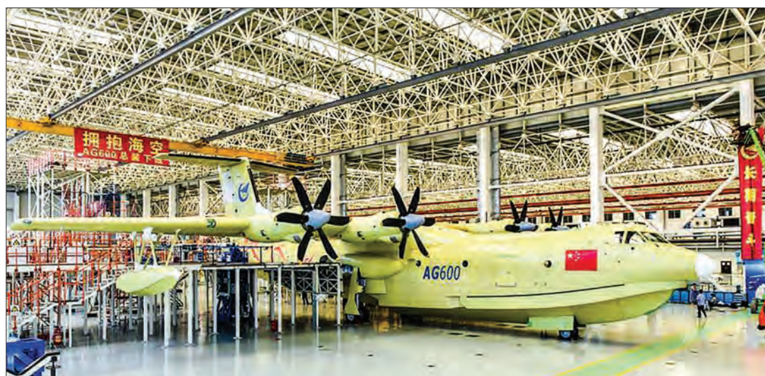
Amphibious aircraft AG600 rolls off a production line in Zhuhai, south China's Guangdong Province, on 23 July 2016. The aircraft, which has a maximum take-off weight of 53.5 tonnes and a maximum flight range of 4,500 km, will be used to fight forest fires and perform marine rescue missions. The AG600 is by far the world's largest amphibian aircraft, about the size of a Boeing 737. PHOTO: XINHUA
