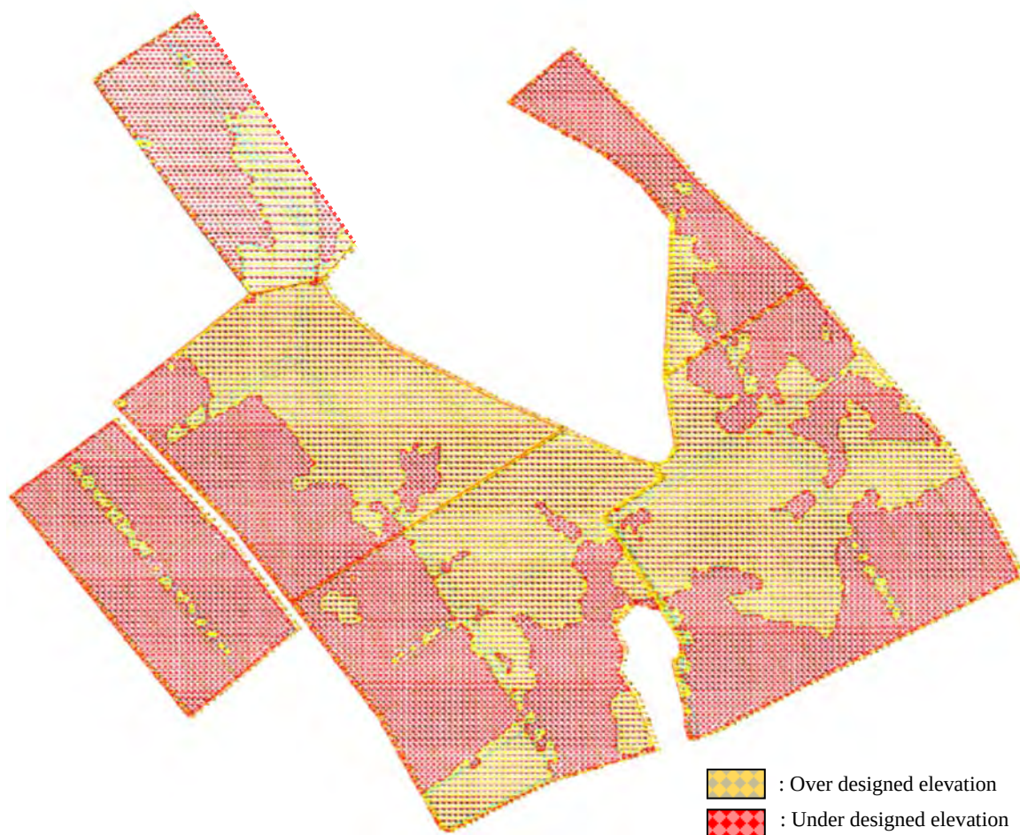
Figure 3.3-1 Land Grading Work of Class A
