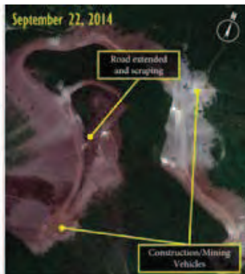
fig 2: Within the mine pit area, imagery shows the road has been extended and significant scraping performed. Many large construction/mining vehicles are visible in imagery from September 22, 2014.
