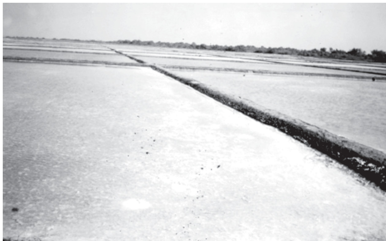
Salt is produced through evaporation of briny water stored in salt pans.
