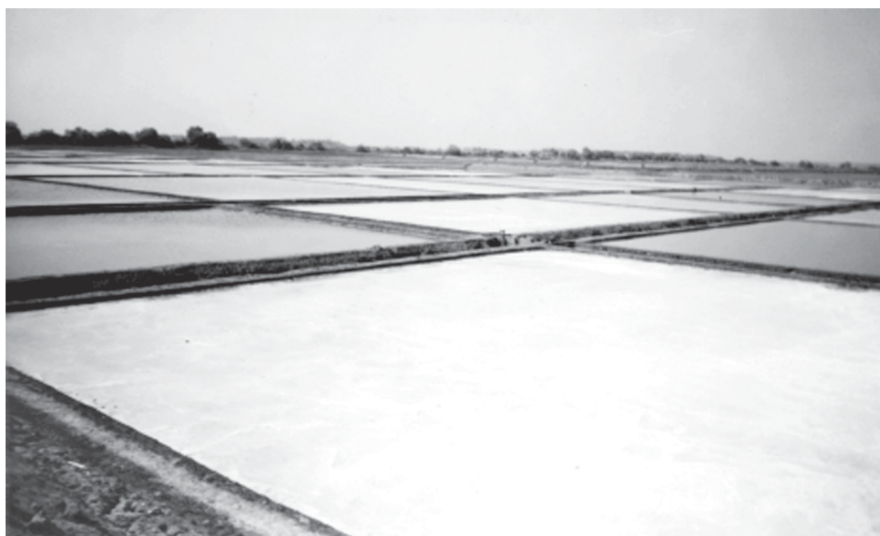
Salt starts to crystalize at 29-degree salinity.
