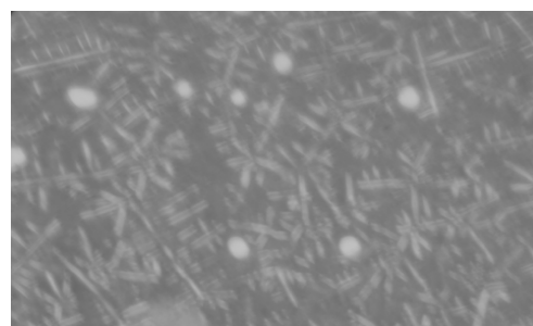
Fig. 1. Photomicrograph of alpha tracks in LR 115 type I for cigarette C 1 sample with 40X objective
