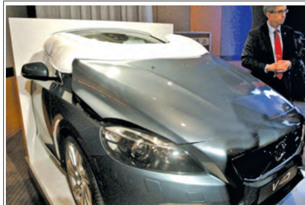
Photo shows the all-new Volvo V40 hatchback featuring the world's first air bag designed to protect pedestrians as Volvo Cars Japan unveiled the vehicle in Tokyo on 19 Feb, 2013.—KYODO NEWS
