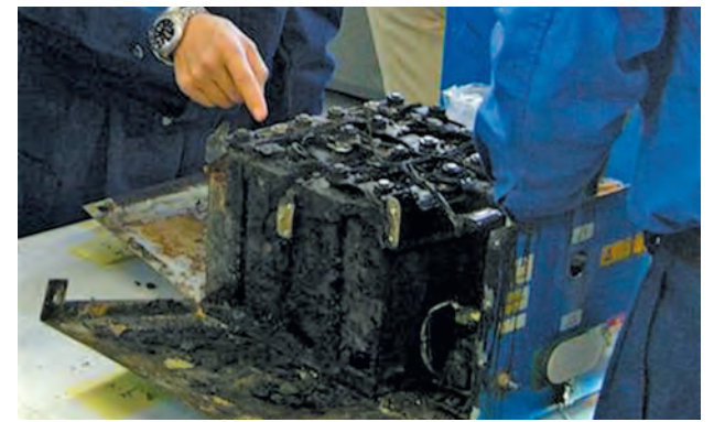
The burnt auxiliary power unit battery, removed from an All Nippon Airways' (ANA) Boeing Co 787 Dreamliner plane which made an emergency landing on 16 Jan, 2013 in Takamatsu, is inspected by the manufacturer at the headquarters of GS Yuasa Corp in Kyoto, western Japan, in this handout photo taken on 26 Jan, 2013 and released by the Japan Transport Safety Board (JTSB) on 5 Feb, 2013.—REUTERS
