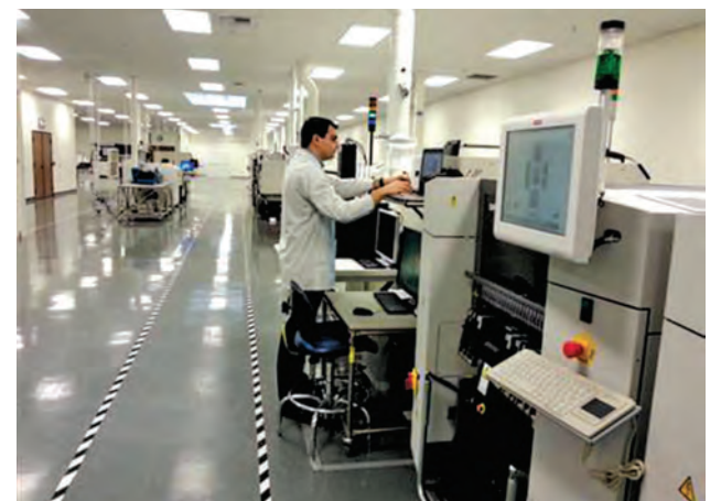
A technician configures a "Pick and Place" electronics manufacturing machine on 11 Feb, 2013 at Flextronics International's Milpitas, California campus. —REUTERS
