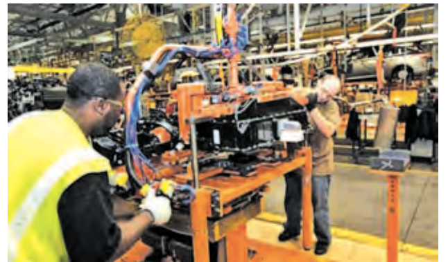
Ford Assembly workers install a battery onto the chassis of a Ford Focus Electric vehicle at the Michigan Assembly Plant in Wayne, Michigan on 7 Nov, 2012.
