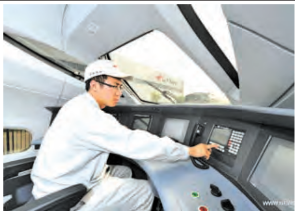
A technician debugs the intelligent control system of China's first intelligent high-speed test train produced by CSR Qingdao Sifang Co, Ltd in Qingdao, a coastal city in east China's Shandong Province, on 27 June, 2013. The test train, with China Railway High-Speed (CRH) 380A train as its technical platform, is China's first large transport vehicle applied with the Internet of Things technology and sensor networks technology, through which passengers could enjoy modern information services like e-ticket and Wi-Fi.
