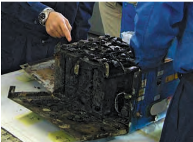
The burnt auxiliary power unit battery, removed from an All Nippon Airways' (ANA) Boeing Co 787 Dreamliner plane which made an emergency landing on 16 Jan 2013 in Takamatsu, is inspected by the manufacturer at the headquarters of GS Yuasa Corp in Kyoto, western Japan, in this handout photo taken on 26 Jan, 2013 and released by the Japan Transport Safety Board (JTSB) on 5 Feb, 2013.—REUTERS
