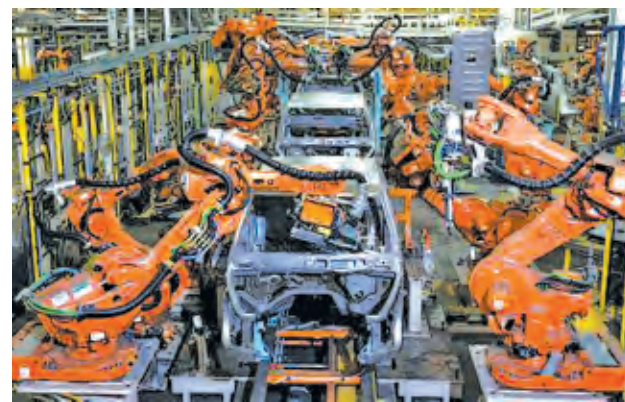
Auto assembly line robots weld on the frame of 2009 Dodge Ram pick-up trucks at the Warren Truck Assembly Plant in Warren, Michigan on 12 Sept, 2008.
