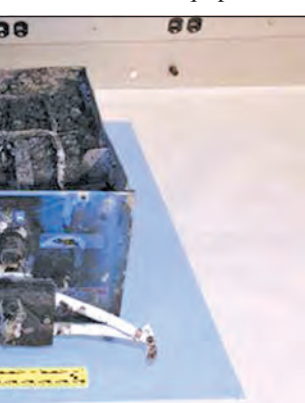
The burnt auxiliary power unit battery removed from a Japan Airlines Boeing 787 Dreamliner jet is seen in this picture provided by the US.—REUTERS
