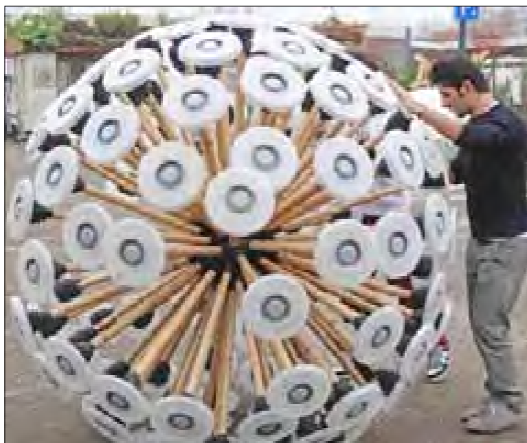
Dutch brothers of Afghan origin Massoud (R) and Mahmud Hassani (L behind round structure) push the 'mine kafon', a wind-driven gadget to clear anti-personnel mines, at their Eindhoven workshop. Pic: AFP
