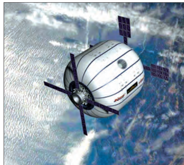
A prototype inflatable space module, developed by Bigelow Aerospace, will be tested aboard the International Space Station.—NHK
