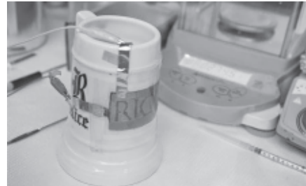
A beer stein served as an able substrate for a paintable battery developed at Rice University.—REUTERS
