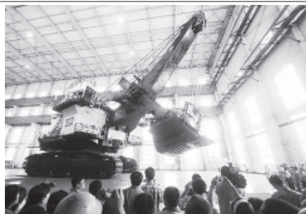
People watch an operation demonstration of the WK-75 mining excavator produced by the Taiyuan Heavy Machinery Group Co, Ltd in Taiyuan, capital of north China's Shanxi Province, on 5 June, 2012. The large equipment, about 37.5 metres in length, 17.3 metres in width and 2,000 tons in weight, is the largest mining excavator in the world. It is capable of digging five million tons of coal in a single month.—XINHUA
