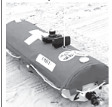
A robot named Emily, which stands for Emergency Integrated Lifesaving Lanyard, are being tested this summer by Los Angeles County, California life-guards as the newest tool to rescue people in water. INTERNET
