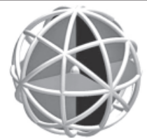
Design for a wind-driven tumbleweed rover.
