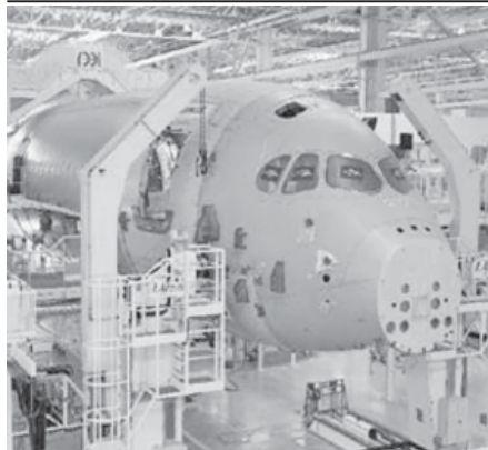
Final assembly of 1st A350 XWB underway in Toulouse, France. This latest step in the A350 XWB's progress was achieved as Airbus started joining the 19.7-meter-long central fuselage with the 21-meter-long front fuselage.
