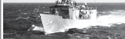
USS Ford (FFG 54) successfully transited from the ship's homeport in Everett, Wash, to San Diego, on 2 March, using 25,000 gallons of a 50/50 algae-derived, hydro-processed algal oil and petroleum F-76 blend in the ships LM 2500 gas turbines. —INTERNET
