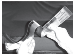
A new sensor was developed for ESA based on super-thin piezoelectric materials that have a special property that converts physical effects like vibration and pressure into minute electric pulses.—INTERNET
