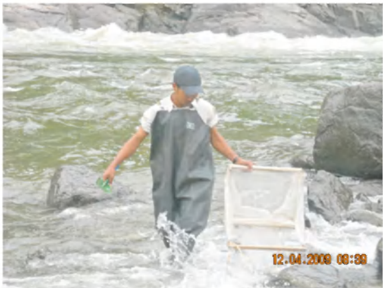
Fig 5.6. Benthos sampling using D-shape kick-net.
