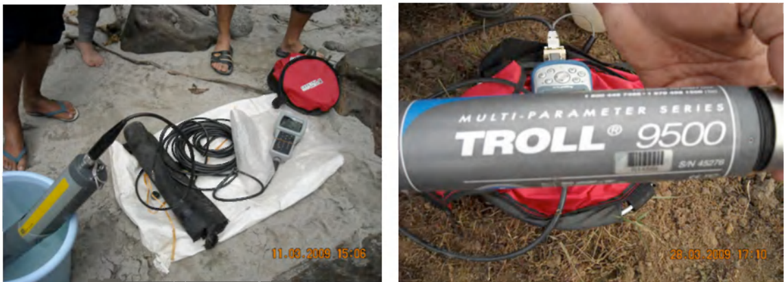
Fig. 5.1. YSI (Yellow Spring Instrument) multipurpose model no. 6600 and TROLL multi-parameter series no. 9500.
