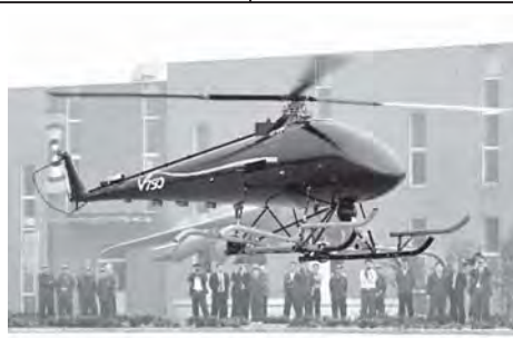
Photo taken on 7 May, 2011 shows the "V750" pilotless helicopter during a test flight in Weifang of east China's Shandong Province. The 757 kilogramme helicopter has a maximum load capacity of 80 kilogramme.
