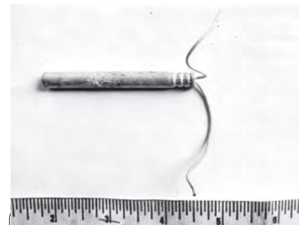
Photo shows an electric detonator with two pieces of wire.
