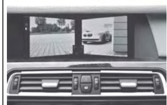
BMW's new Multicamera System can give you a valuable look forward when entering tricky intersections.—INTERNET
