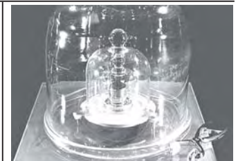
The original cylinder of platinum and iridium used as the standard weight for one kilogramme. Scientists said Monday they were moving closer to coming up with a non-physical definition of the kilo after discovering the metal artefact used as the international standard had shed a little weight.
