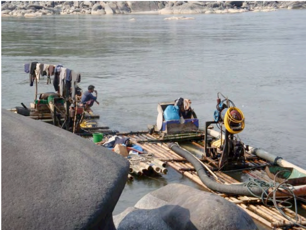
Fig. 11 Suction dredging on the Mayhka
