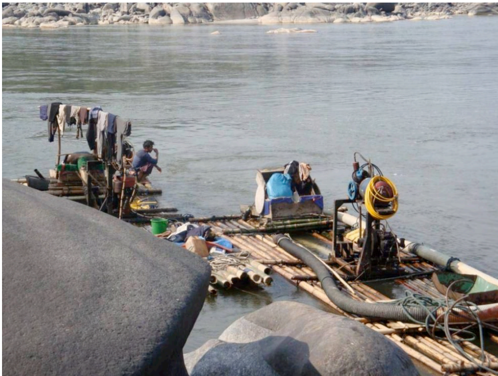
Fig. 11 Suction dredging on the Mayhka
