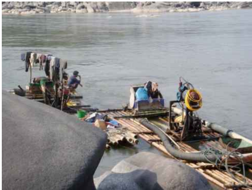
Fig. 11 Suction dredging on the Mayhka
